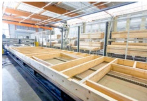
transport of the wooden frames between cells by roller conveyors
