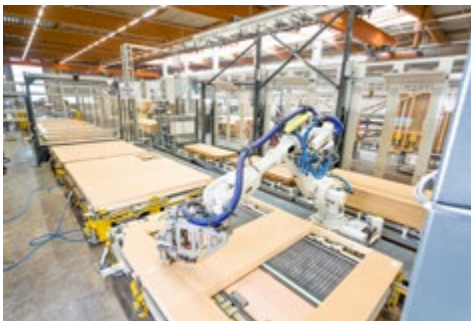
staples on the sheets with defined staple tracks and corners
