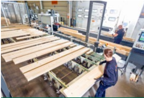
positioning of the cut sections for the wooden frame by semi-automatic feed conveyor
