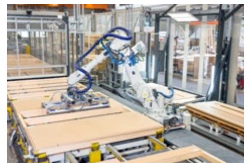
fast transfer of data to robot with vacuum gripper for precise paneling with timber sheets
