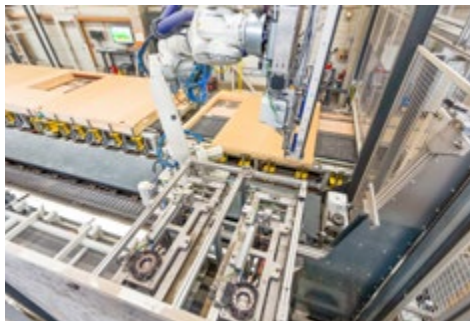
gripper changeover from stapler to vacuum gripper
