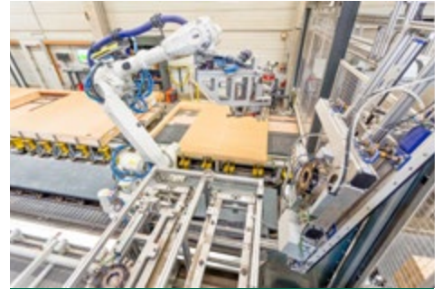
automatic robot gripper change from vacuum gripper to stapler
