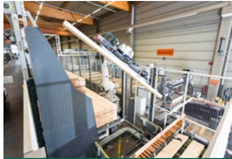
provision of the standard lengths of timber by robot from magazines
