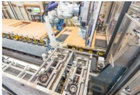
gripper changeover from stapler to vacuum gripper
