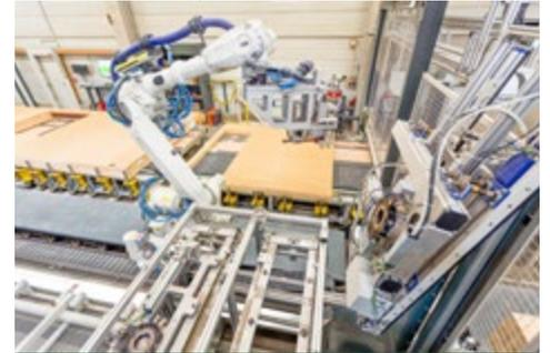
automatic robot gripper change from vacuum gripper to stapler
