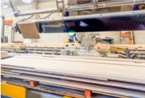
detection and removal of filler pieces required for processing
